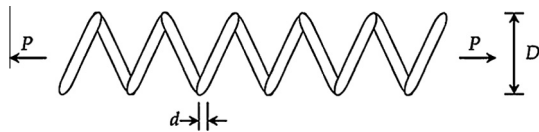
Fig. 8. Schematic of tension/compression spring design problem.
